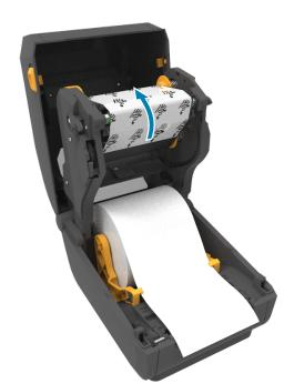
Pull the supply ribbon leader up and over the printhead and attach it to the take-up spool.
