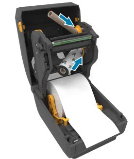
Push the right side of the spool onto the spring-loaded spindle.
