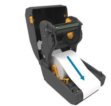
Pull the end of the roll past the front edge of the printer.
